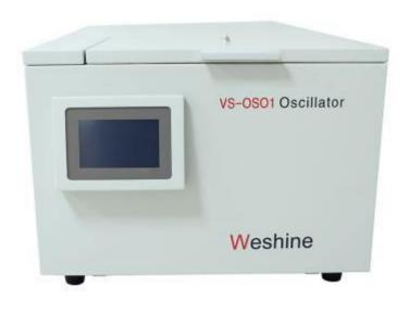
The Oscillator heats and shocks the transformer oil to extract the gases from the transformer insulating oils automatically. The temperature and times can be set. Put the 40ml oils into the 100ml-injector, and then put 8 injectors at max into the oscillator to start the extraction works.
