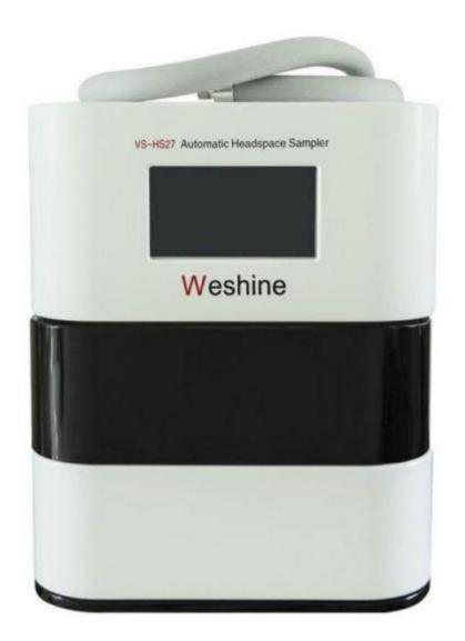
The Autosampler can extracts the gases from the insulating oils, and transmit the gases by carrier gas to the **Headspace Gas Chromatography** Columns. It has the function of the heating and shocking, instead of the manual oscillator.
