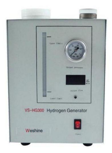
This Hydrogen Generator make the hydrogen for the **Online Gas Chromatography**, the hydrogen can help to fire the FID1 and FID2.
